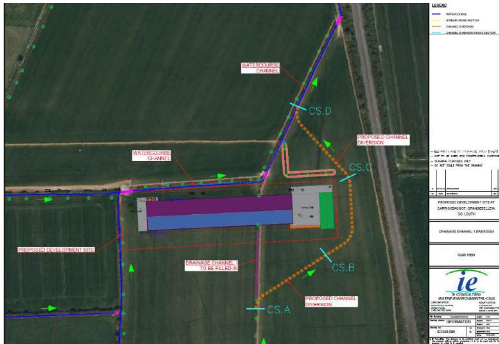
Fig 7.3 c- detaining the option of an open diversion drain.
