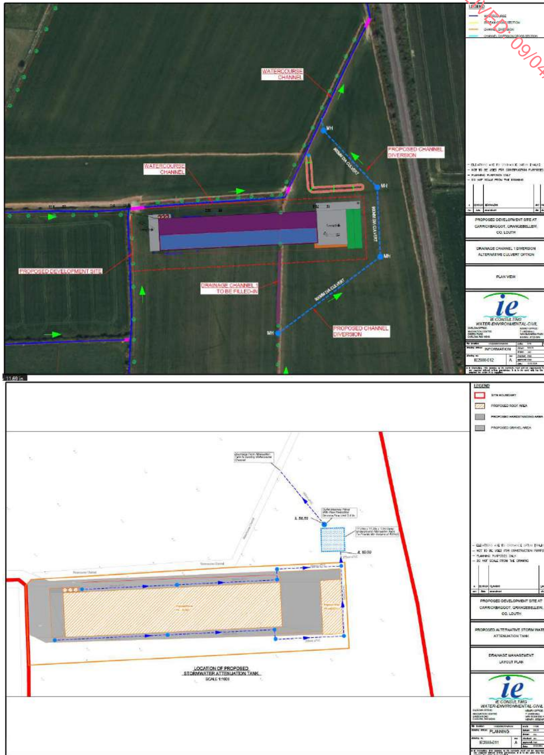
Fig: 7.3 a and b detailing both stormwater attenuation options (Open Swale, or enclosed tank)
